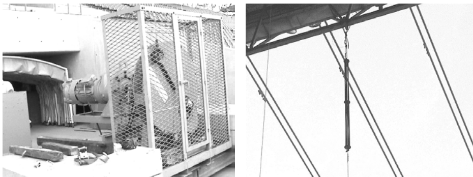
Figure 2. View of the electric engine with the eccentric link (left) and of the girder linked spring (right).
