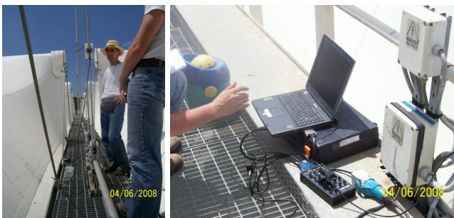
Figure 4: Dynamic measurement of natural frequencies for the force determination
