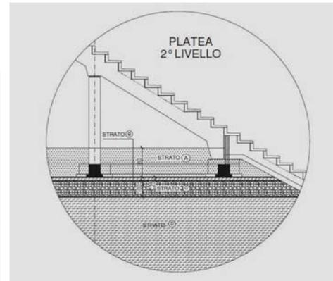
The foundation system is based on a texture of direct beams foundation on ground stratification with different characteristics:
