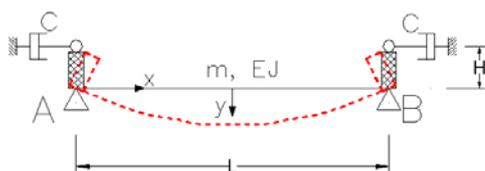
Figure 2. Scheme of the simply supported beam with end-located dampers.
