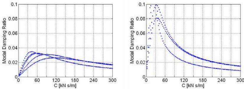
Figure 8. Modal damping ratio of first 5 modes for the case (a)  $C_1 = 0$  to 300 kN s/m and (b)  $C_3 = 0$  to 300 kN s/m.
