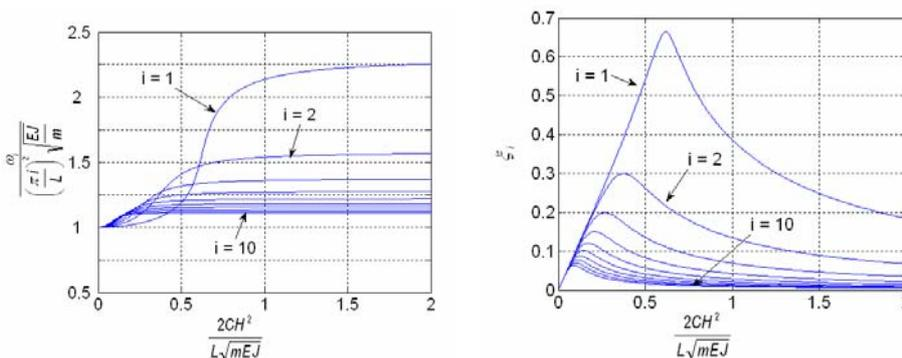
Figure 4. Modal frequency and modal damping ratio of the first 10 real modes for different values of the damping coefficient.
