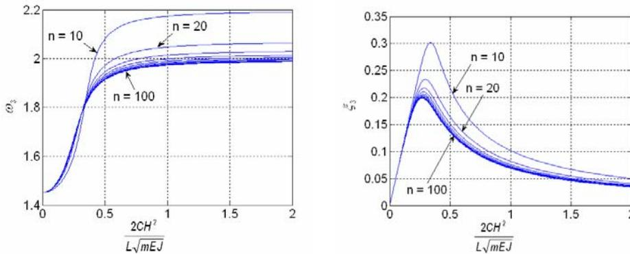
Figure 3. Numerical convergence of modal frequency and damping ratio of the 3<sup>rd</sup> mode by using different undamped modes.
