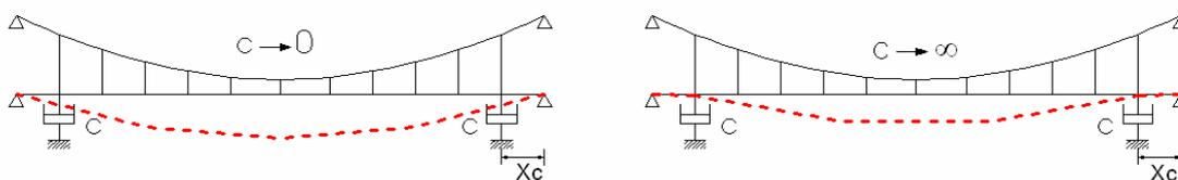
Figure 1. The existence of an optimal damping value for flexible structures.
