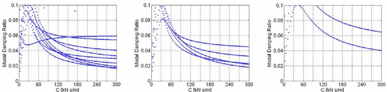
Figure 9. Modal damping ratio of first 20 modes for  $C_3 = 0$  to 300 kN s/m and (a)  $C_d = 18$  kN s/m, (b)  $C_d = 30$  kN s/m and (c)  $C_d = 240$  kN s/m with a stiffened deck girder.
