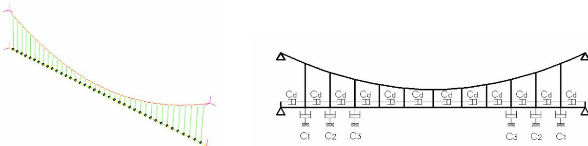
Figure 5. Scheme of (a) the FEM model used for the modal analysis and (b) the four considered damper arrangements.
