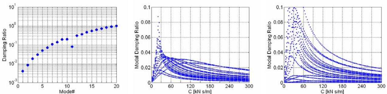
Figure 7. Modal damping ratio of first 20 modes for (a)  $C_d = 60 \text{ kN s/m}$ ; (b)  $C_1 = 0$  to  $300 \text{ kN s/m}$  and (c)  $C_3 = 0$  to  $300 \text{ kN s/m}$ .
