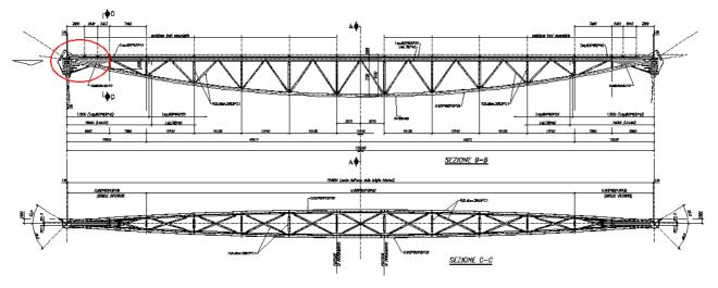
Main truss with terminal suspending joint
