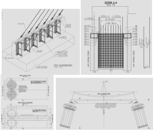
These are the foundations of the two legs main columns, are made with two deep wells made of jet
