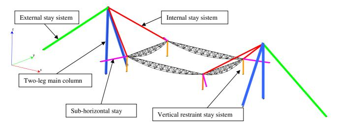
Each leg of main column has tapered shape. Cross section shape is triangular formed by 3 curved plates 30/35mm thick. In the middle span the triangle side is about 3.75m length.
